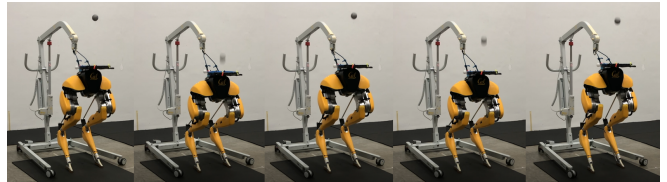
Fig. 1. Snapshots of experiments on the Cassie-paddle-ball system. Two juggles, shown here, take 0.6 sec per bounce on average. Experimental videos are accessible at https://hybrid-robotics.berkeley.edu/cassie-juggling .
