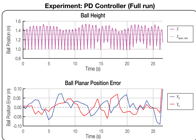
Fig. 6. Experimental results for a 42-bounce run. The peak planar position error was 7 cm, well within the confines of the racket, and the average apex overshoot was 13.8 cm. The spike in planar error corresponds to the failure mode of this run: the ball hit the frame of the racket and bounced off.
